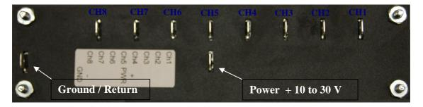
The positive power input is identified as the center spade on the back. While the negative power input (ground or return) is identified as the far left side spade. The eight channel load ports are along the top.
