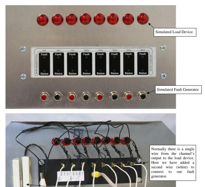
We can bridge across the load either 1 or 2 Ohms to induce an extra 14 or 7 amps of load current.
